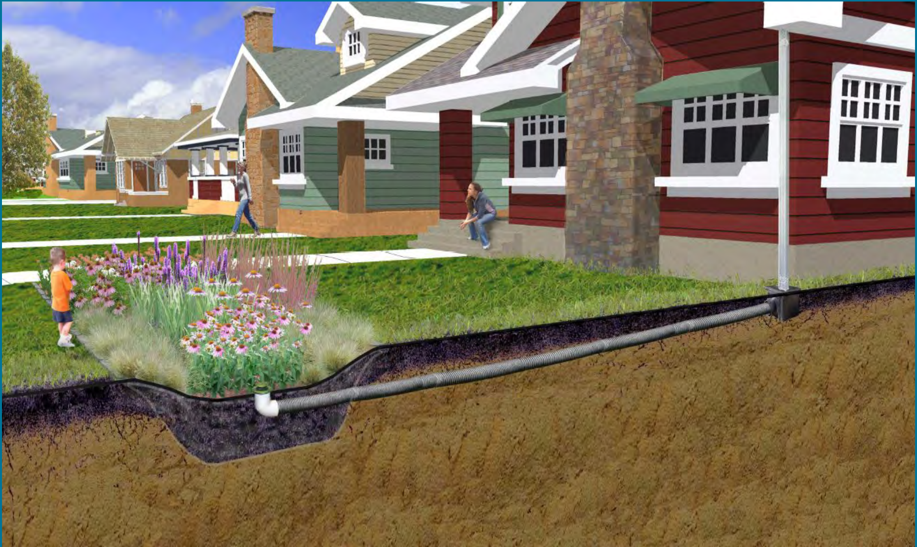
Raingarden with downspout connection
